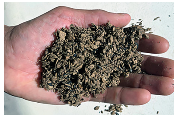
Municipal solid waste fiber following the Hughes process. Additional processing will transform it for use in a variety of consumer products.
