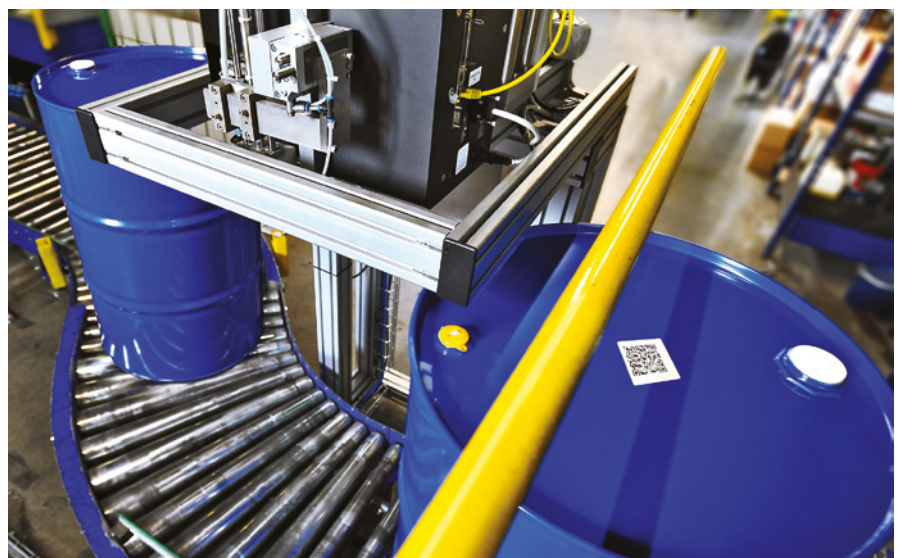
The QR code on the lid of the vat contains all the important information about the product (Herma).
