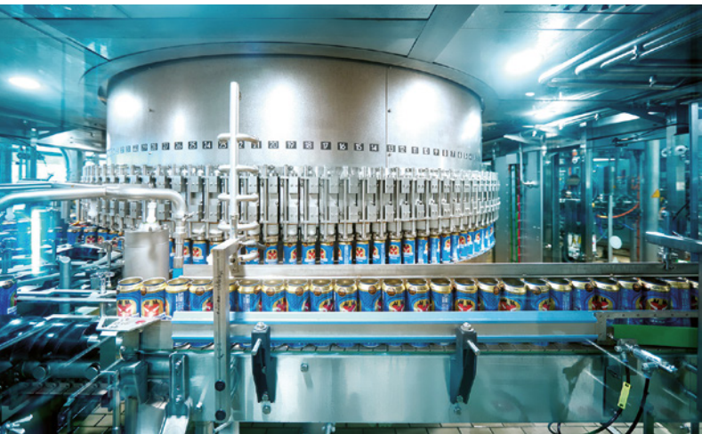
Filler and seamer part of the combined block solution SmartCan by KHS/Ferrum feature optimised hygienic properties. Copyright: Roth und Schmid Fotografie
