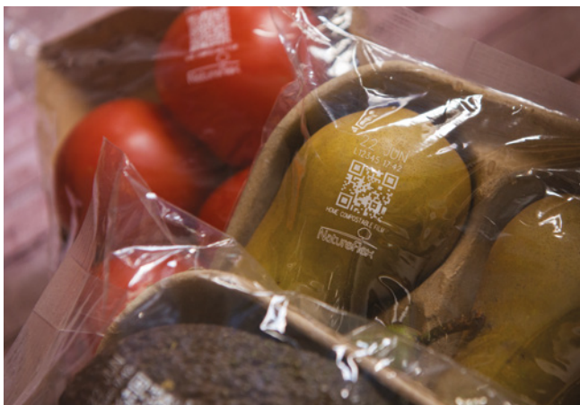
Crisp and clear: QR code applied by laser to a compostable film (Domino Germany).
